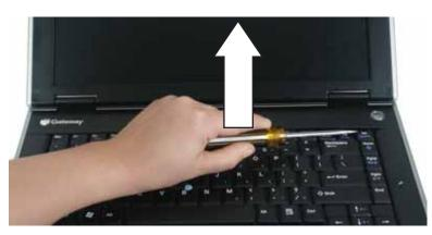
**12** Pull the cover off the notebook. Be careful to not damage the LCD panel.
